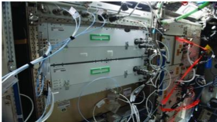
Figura 48. Spaceborne Computer-2 de Hewlett Packard Enterprise en la ISS. Fuente: https://spacenews.com/booz-allen-deploys-advanced-language-model-in-space/
